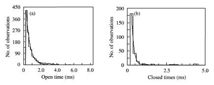
FIG. 2. Dwell time distributions to +40 mV for the channel shown in Fig. 1. (a) represents the open time and (b) the closed time distribution. The lines represent best fits of exponential functions to the experimental data points, using the Levenberg Marquardt algorithm. Number of events is 2330. Note that the histogram for the closed times has the abcissa expanded in order to better visualize the fitting. The exponentials are described in the text.
