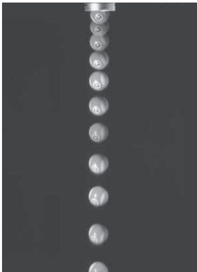
FIGURE 2.11 Strobe photo of a falling ball. Successive images are farther apart, showing that the ball is accelerating.
