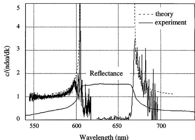
Fig. 4. Ratio of RCP to LCP emission spectra from sample 2 and theoretical curve for  $(c/n)/(d\omega/dk)$  for the stop band.
