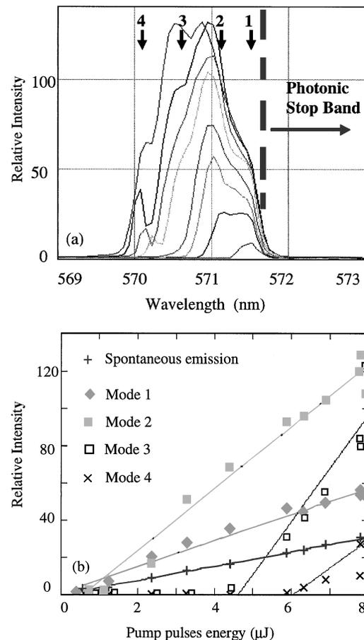
Fig. 2. (a) Emission spectrum with peaks at wavelengths 1–4 from sample 1 at different pump powers. (b) Relative intensities of emission at the wavelength corresponding to each mode.
