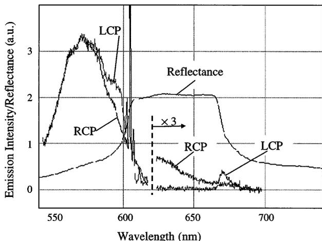
Fig. 3. Emission spectra from sample 2 for LCP and RCP emission with the reflectance spectrum superimposed.
