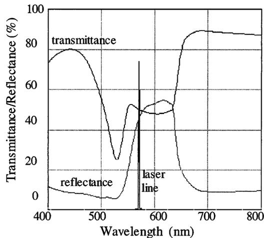
Fig. 1. Transmittance and reflectance spectra for unpolarized light of dye-doped CLC for sample 1 with superimposed laser emission.
