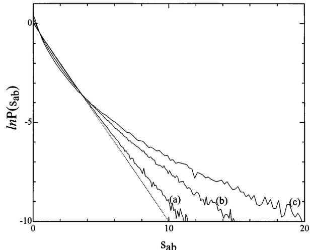
Fig. 2. Measured intensity distributions for three samples: (a)  $L = 67$  cm,  $d = 7.5$  cm,  $L/\xi \approx 1/15$ ; (b)  $L = 200$  cm,  $d = 5$  cm,  $L/\xi \approx 2/5$ ; (c)  $L = 520$  cm,  $d = 5$  cm,  $L/\xi \approx 1$ . The Rayleigh distribution is represented by the dotted line.
