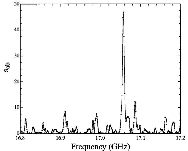
Fig. 1. Intensity spectrum for a single sample configuration for the sample with  $L = 520$  cm ( $\approx \xi$ ) and  $d = 5$  cm.
