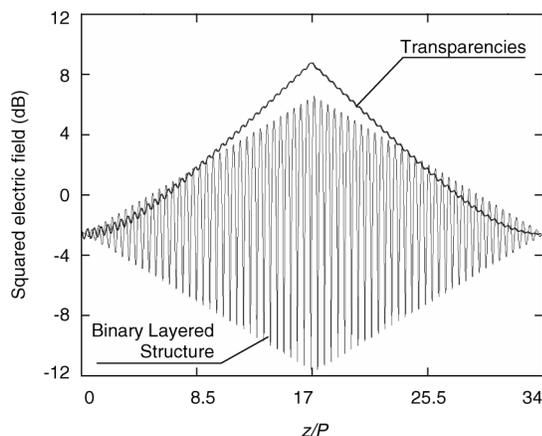
Fig. 4. Comparison of the energy density inside chiral and binary layered structures with the same index contrast and thickness versus coordinate  $z/P$ . Pitch  $P$  of the chiral structure is twice the period of the binary-layered structure.
