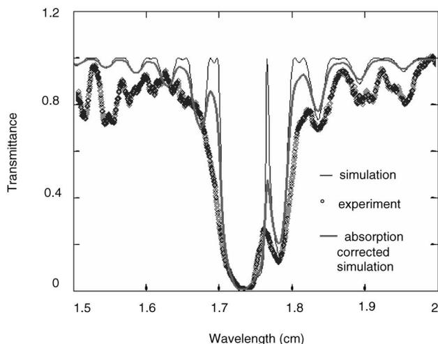
Fig. 5. Transmittance through a stack of 3000 transparencies with a  $45^\circ$  chiral twist in the center.
