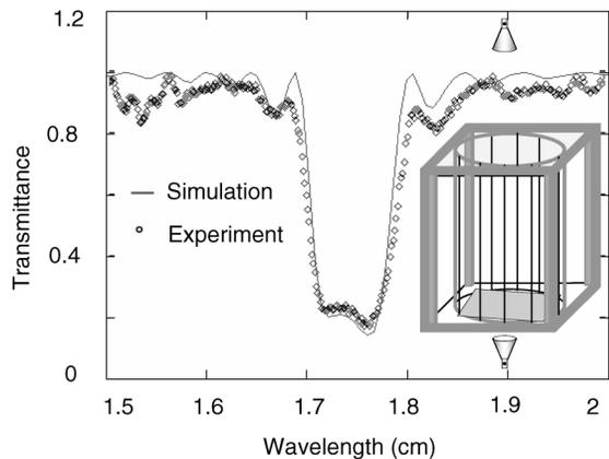
Fig. 1. Transmittance through a stack of 1500 transparencies.
