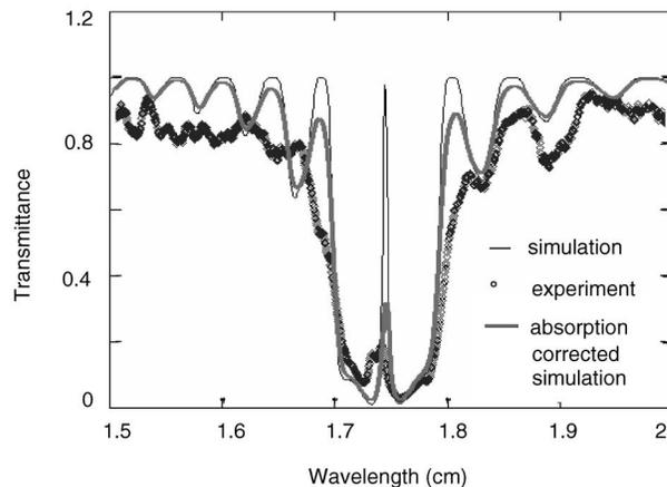
Fig. 2. Transmittance through a stack of 3000 transparencies with a  $90^\circ$  chiral twist in the center.
