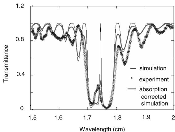
Fig. 6. Transmittance through a stack of 3000 transparencies, with a combination of a  $45^\circ$  chiral twist and a quarter-wavelength separation in the center.
