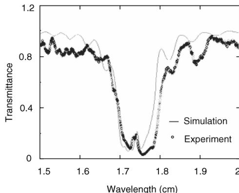
Fig. 3. Transmittance through a stack of 3000 transparencies with a  $90^\circ$  chiral twist in the center. Both angular spread and absorption are taken into account in the simulation.
