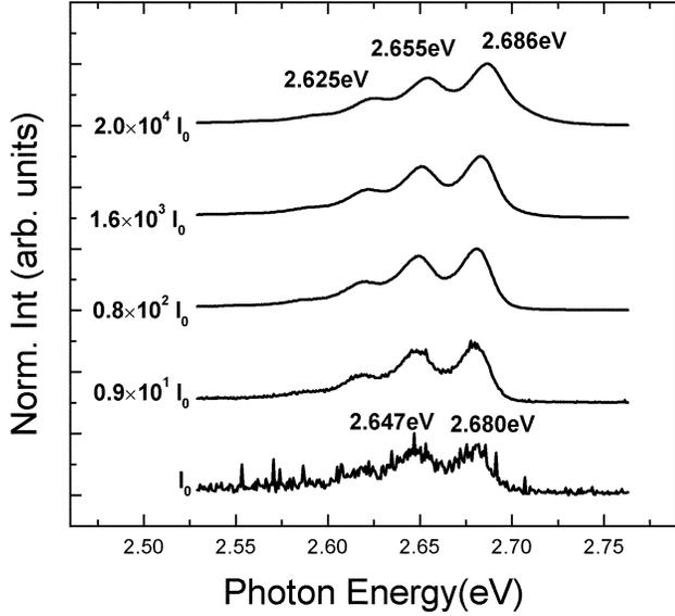
Fig. 1. The PL spectra of sample A at different excitation intensities.
