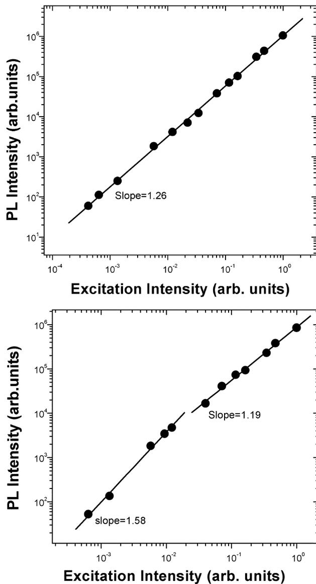
Fig. 4. The integrated PL intensity as a function of laser-excitation intensity: (a)  $\delta$ -doped ZnSe:Te, N and (b)  $\delta^3$ -doped ZnSe:(Te, N).
