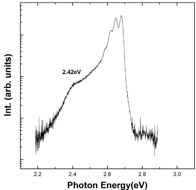
Fig. 3. The PL spectra of sample A at low-excitation intensity.
