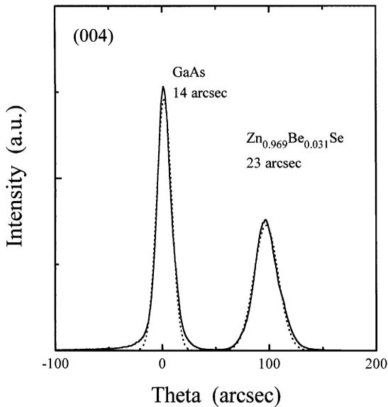
Fig. 1. (004) reflection DCXRC for an undoped  $\text{Zn}_{0.969}\text{Be}_{0.031}\text{Se}$  layer grown after Be–Zn co-irradiation of the GaAs surface. The solid line is the experimental data and the dotted line is the Gaussian fit.
