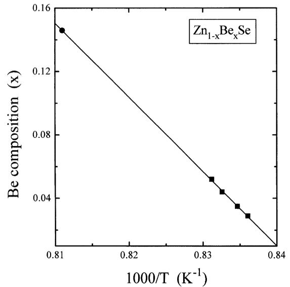
Fig. 2. Dependence of Be composition of  $\text{Zn}_{1-x}\text{Be}_x\text{Se}$  alloys on the Be cell temperature during growth. Squares were calculated from the (1 1 5) *a* and *b* reflection DCXRC, and the circle was calculated from the (0 0 4) reflection single crystal XRD data assuming that the epilayer is completely relaxed.
