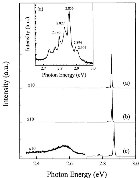
Fig. 3. Low-temperature (13 K) PL spectra for undoped ZnBeSe layers grown using (a) Be–Zn co-irradiation with a ZnSe buffer, (b) a BeTe buffer and (c) Zn-irradiation with a ZnSe buffer. The inset is the semi-log plot near the band gap region of spectrum (a).
