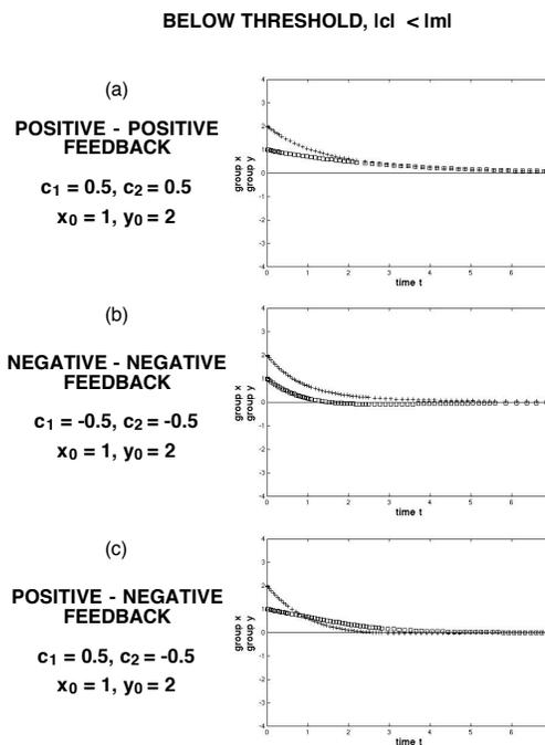
Figure 2: Numerical integration was used to compute the values of  $x$  (boxes) and  $y$  (plus signs) as the state of the two groups evolves from their initial values of  $x = 1$  and  $y = 2$ . When the strength of the feedback is less than the absolute value of the inertia to change, then all the models evolve to the neutral state  $x = 0$  and  $y = 0$ .
