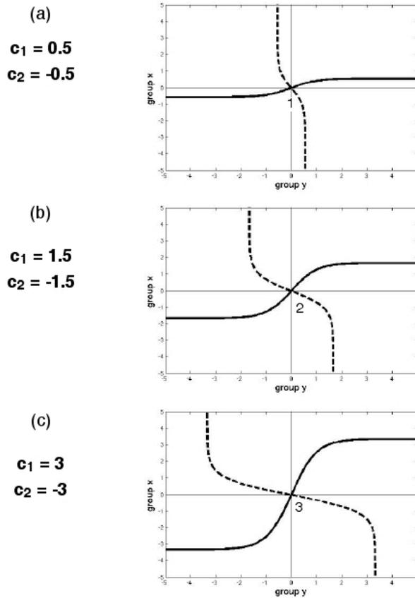
Figure 8: The intersection of the nullclines for  $dx/dt = 0$  (solid line) and  $dy/dt = 0$  (dashed line) for positive-negative feedback between the groups determine the critical points. The stability of these critical points is evaluated in the Appendix. For all strengths of the feedback there is only critical point (1,2,3) which is stable.
