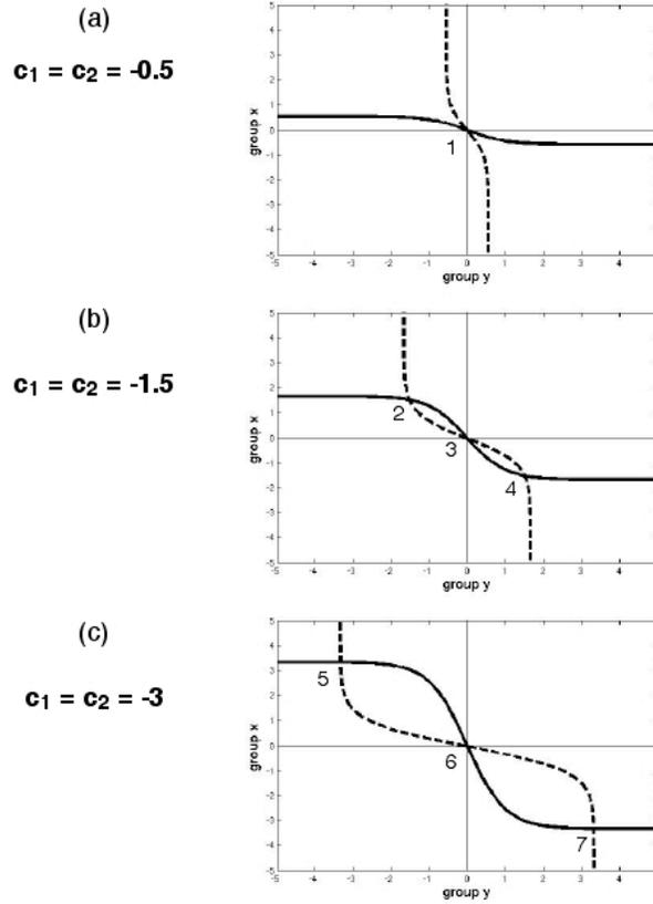
Figure 5: The intersection of the nullclines for  $dx/dt = 0$  (solid line) and  $dy/dt = 0$  (dashed line) for negative feedback between both groups determine the critical points. The stability of these critical points is evaluated in the Appendix . (a) When the strength of the feedback is weak there is only one fixed point (1). (b,c) As the strength of the feedback increases two new fixed points (2, 4 and 5, 7) appear and the original critical point (3, 6) becomes an unstable saddle.
