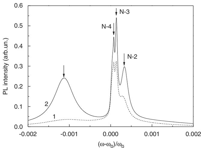
Fig. 1. Calculated PL spectra for a near-Bragg MQW structure (1) with semi-infinite barriers and (2) with one semi-infinite barrier and a finite cap layer of thickness  $b' = d - (a/2)$ . The structure parameters chosen are as follows: the number of QWs  $N = 100$ ,  $d/\lambda(\omega_0) = 0.495$ ,  $\hbar\omega_0 = 1.5$  eV,  $n_a = n_b = \sqrt{13}$ ,  $\hbar\Gamma_0 = 27$   $\mu$ eV, and  $\Gamma = \Gamma_0$ . Arrows indicate real parts of four exciton–polariton eigenfrequencies.
