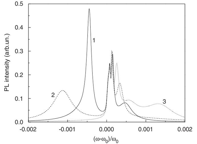
Fig. 2. Effect of the dielectric contrast on the PL spectral shape from the near-Bragg MQW structure with 100 wells and the cap layer of thickness  $b' = d - (a/2)$ . Curves 1–3 are calculated for the QW background refractive index given by  $n_a/n_b = 0.9; 1$  and  $1.1$ , respectively. Other parameters coincide with those indicated in the caption to Fig. 1.
