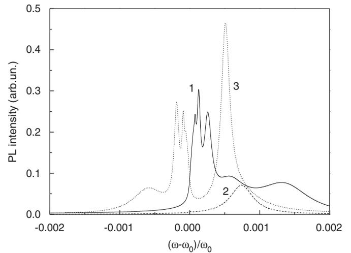
Fig. 3. Variation of the PL spectra with the period of the MQW structure containing 100 wells. Curves 1–3 are calculated for  $d/\lambda(\omega_0) = 0.495, 0.5$ , and  $0.505$ , respectively, and the cap layer of the thickness  $b' = d - (a/2)$ . Other parameters coincide with those indicated in the caption to Fig. 1.
