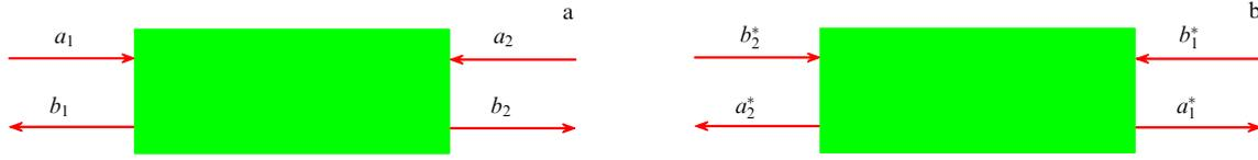
**Figure 7.** (a) Schematic representation of the scattering of plane waves from a one-dimensional optical system:  $a_i$  are the complex amplitudes of waves incident on the system,  $b_i$  are the complex amplitudes of waves scattered by the system. (b) Schematic representation of the scattering of plane waves from a one-dimensional optical system, shown in Fig. 7a, after its  $\hat{P}\hat{T}$  transformation.
