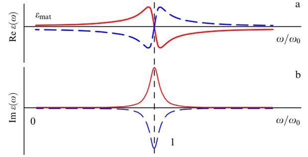
**Figure 1.** (a) Real and (b) imaginary parts of the permittivity for absorbing (solid curves) and gain (dashed curves) media in the case where imaginary parts differ only in sign:  $\text{Im} \varepsilon_{\text{loss}} = -\text{Im} \varepsilon_{\text{gain}}$ .
