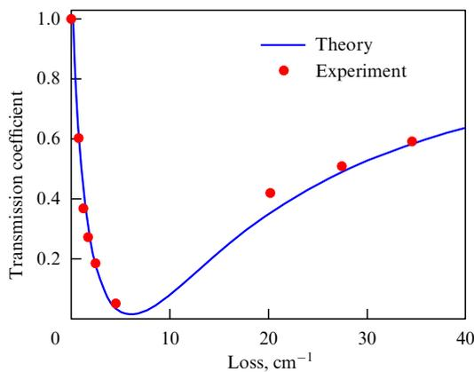
**Figure 5.** Transmission coefficient for light propagating through a system of two coupled waveguides as a function of the loss in the second waveguide [49].
