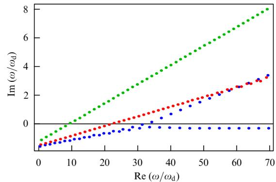
**Figure 9.** (Color online.) Position of poles of the scattering matrix in the complex frequency plane. The real part of the frequency is plotted on the abscissa and the imaginary part of the frequency  $\text{Im}(\omega/\omega_d)$ , where  $\omega_d = \pi c/(2d)$  on the ordinate axis. Green, red, and blue colors respectively indicate system poles with  $\alpha = 1.0, 0.5$ , and  $0$ .
