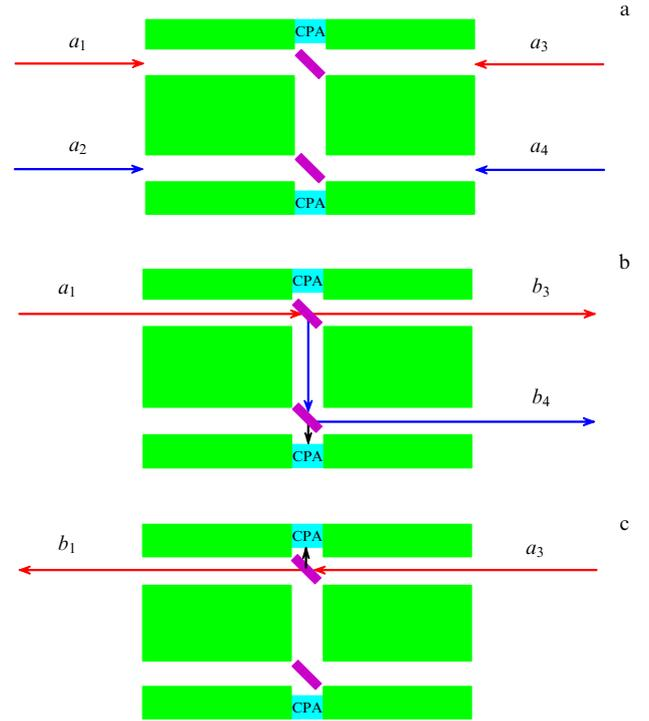
**Figure 14.** (a) Schematic representation of the scattering of waves from an optical system (notation as in Fig. 12a). (b) Schematic of the incidence of the even mode on the system from the left. (c) Schematic of the incidence of the even mode on the system from the right. The inclined rectangles are semi-transparent mirrors. CPA is a coherent perfect absorber. The situation is completely analogous to that for the scattering of waves by a PT-symmetric system.
