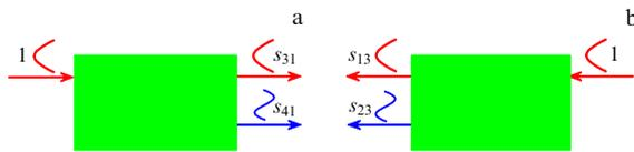
**Figure 13.** Schematic representation of the incidence of the even mode with the unit amplitude on the system (a) from the left and (b) from the right.
