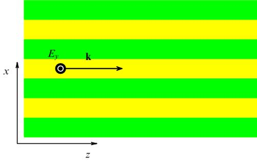
**Figure 2.** Two-dimensional PT-symmetric optical systems,  $\varepsilon(x, z) = \varepsilon^*(-x, z)$ . Different values of the permittivity are indicated by different colors; the arrow shows the propagation direction of electromagnetic waves.
