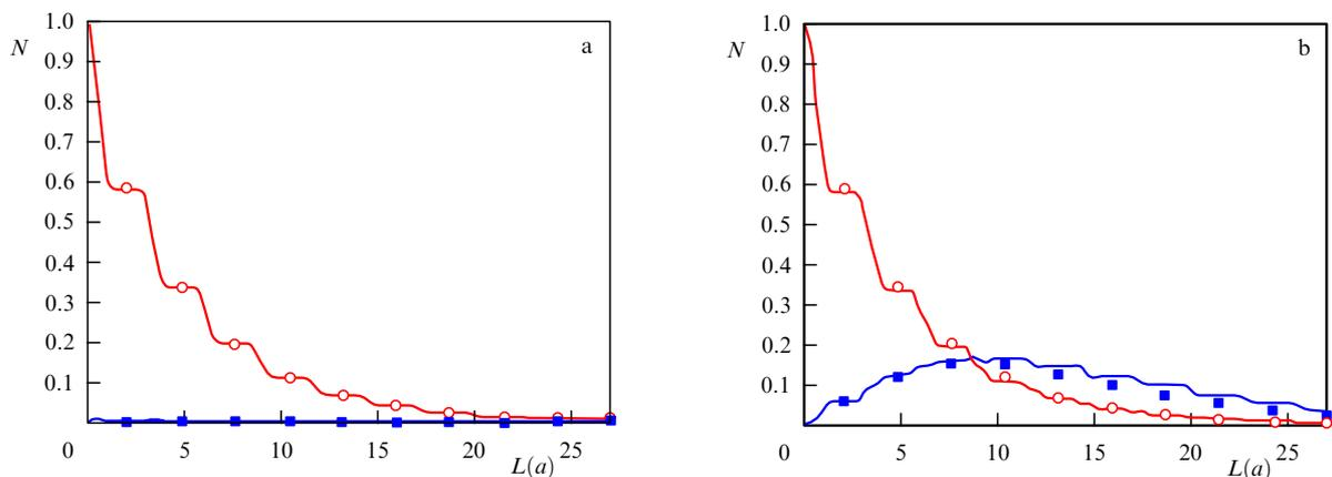
**Figure 11.** (Color online.) (a) Amplitudes of the even (red) and odd (blue) modes upon the incidence of the even mode from the left on the system, as a function of the system thickness. (b) Amplitudes of the even (red) and odd (blue) modes upon the incidence of the even mode from the right on the system, as a function of the system thickness. (From Supporting Online Material in [63].)
