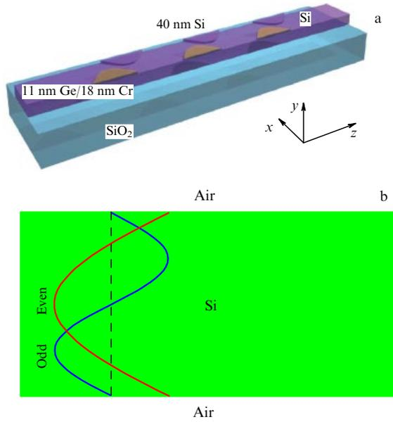
**Figure 10.** (Color online.) (a) Diagram of a PT-symmetric optical system of two coupled rectangular waveguides PT-symmetric along the  $z$  axis. (b) Field distributions in the even (red curve) and odd (blue curve) modes of the PT-symmetric optical system shown in Fig. 10a [62].
