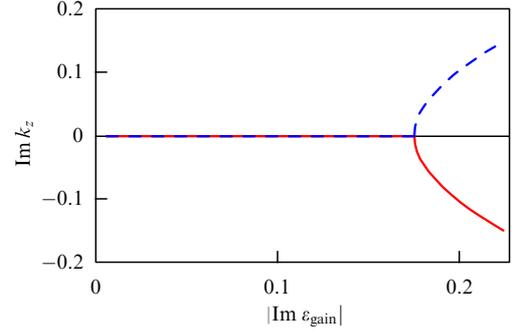
**Figure 3.** Dependence of the imaginary part of the effective wave vector on the imaginary part of the permittivity for  $k_0 d = 10\pi$ .
