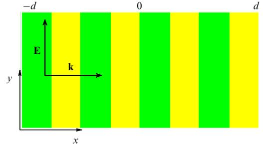
**Figure 6.** (Color online.) One-dimensional PT-symmetric optical systems,  $\varepsilon(x) = \varepsilon^*(-x)$ . Different values of the imaginary part of the permittivity are shown by green and yellow colors. The vector  $\mathbf{E}$  shows polarization and the vector  $\mathbf{k}$ , the propagation direction of an electromagnetic wave.
