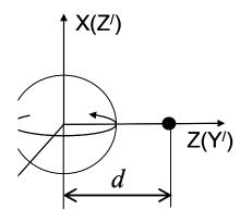
FIG. 1: The coordinate systems used in calculations. The curved arrow schematically represents the counterclockwise fundamental mode whose interaction with the defect (blackened small sphere) is under consideration.
