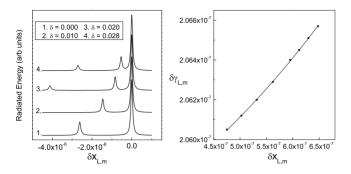
FIG. 2. Scattered power for different distance parameter  $\delta = (d - R_0 - R_d)/R_0$  (left); relative broadening versus frequency shift of the |m| = 1 resonance revealed through varying distance d (right). The line shows a fit with a quadratic polynomial.
