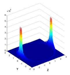
FIG. 3. (Color online) Internal field intensity of the microsphere in the YZ plane at the frequency of the standard Mie resonance (left) and the defect-induced resonance (right).
