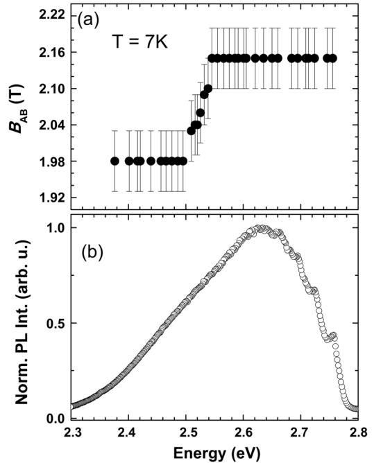
FIG. 2. (a) Spectral dependence of  $B_{AB}$ ; (b) PL spectrum. Note the high energy shoulders in (b) are seen as sharp lines in higher resolution measurements shown in Fig. 1.
