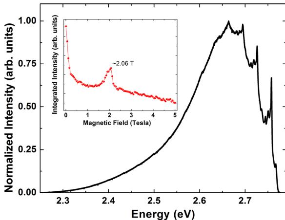
FIG. 1. Low temperature ( $T = 10$  K) high resolution PL of type-II QD sample grown with three Zn-Te-Zn sequences. Inset: integrated PL intensity as a function of magnetic field; the peak at 2.06 T is due to the excitonic AB effect.
