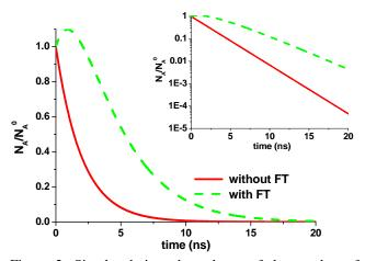
Figure 2: Simulated time dependence of the number of excitons in acceptors. The main panel (linear scale) demonstrates the characteristic increasing of the number of excitons in acceptors when QDs are coupled with the Förster transfer, whereas the inset (in logarithmic scale)
