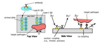
Figure 3: Illustration of the pathogen-sensing platform in gaseous environment.
