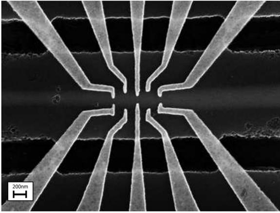
FIG. 1. A micrographic image of the suspended nanobridge with patterned gate pairs that form five QPCs. The interdigitated transducers (IDTs) that generate the SAW are located on either side of this structure (not shown due to the scaling).
