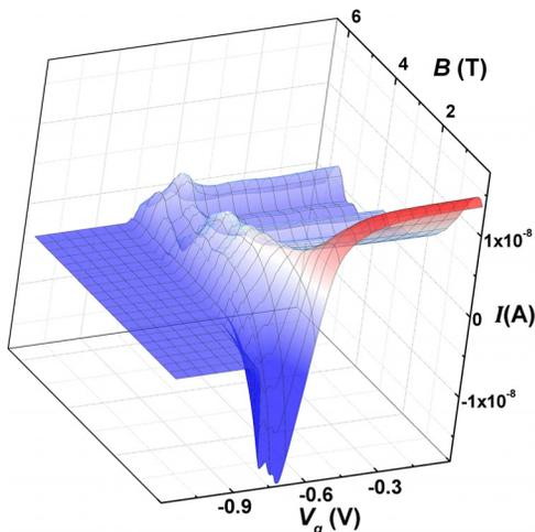
FIG. 2. Dependencies of acoustoelectric current on the QPC gate voltage and the magnitude of the magnetic field.
