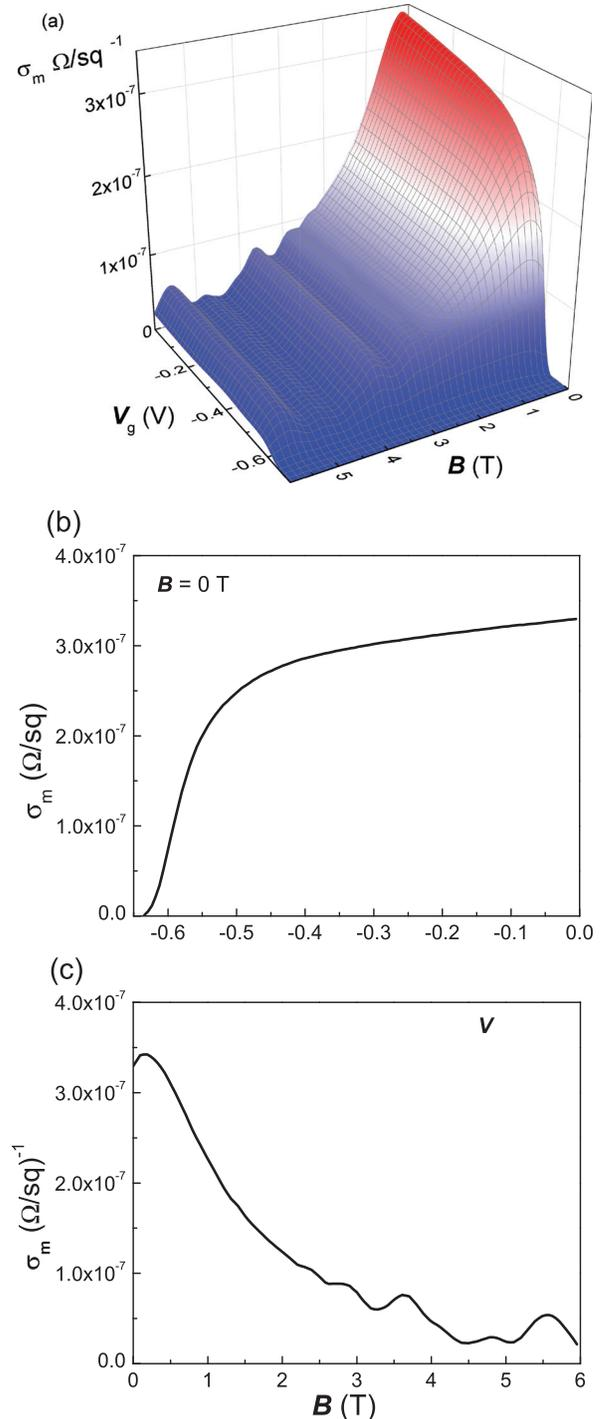
FIG. 3. (a) Dependencies of  $\sigma_m$  on the QPC gate voltage and the magnitude of the magnetic field. (b) Dependence of  $\sigma_m$  on the gate voltage for the zero magnetic field. (c) Dependence of  $\sigma_m$  on the magnetic field for zero gate voltage.
