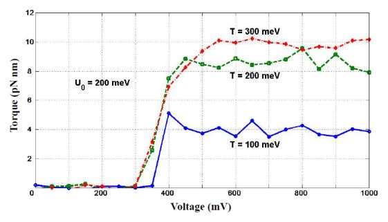
Fig. 5. Dependence of the time-averaged torque on the source-drain voltage.
