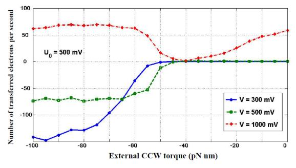
Fig. 6. Dependence of the particle current on the external counterclockwise (CCW) torque.
