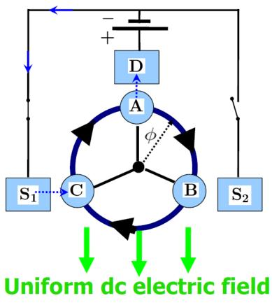
Fig. 1. Schematics of the nanomotor. With  $S_1$ -lead connected to the circuit, the rotor experiences the clockwise rotation. The Hamiltonian of the system has the form:
